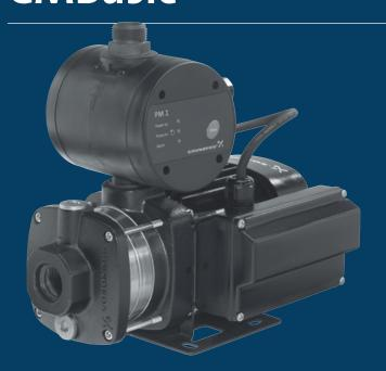
The Grundfos CMBasic is a compact booster pump designed for domestic and light industrial use. The booster unit consists of a Grundfos CM cast iron pump with stainless steel hydraulic components and PM1 Pressure Manager. The Pressure Manager allows the pump to start and stop automatically according to demand and protects the pump from dry running.
